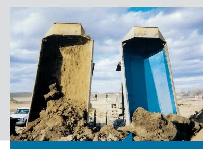
A worn truck bed makes unloading ever more time-consuming and more dangerous, because the load only starts to slide at extreme angles.
